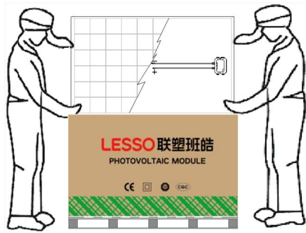
Figure 2 Removing PV modules from a pallet
